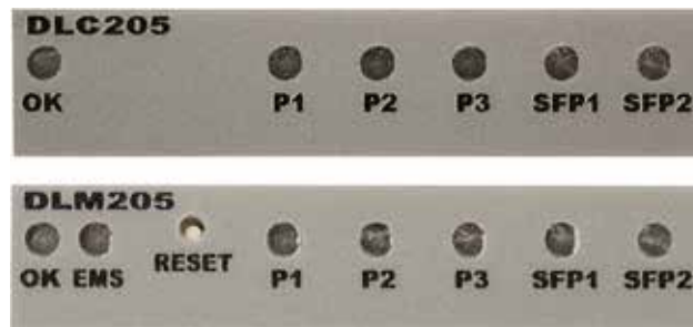
Figure 6. DLC205/DLM205 Front Panel Status LEDs
