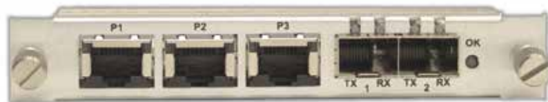
Figure 7. DLC205/DLM205 Rear Panel Status LEDs
