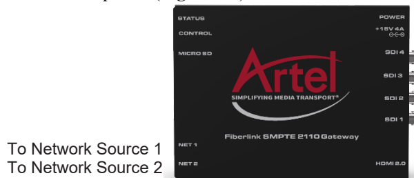
Figure 5.1 FL ST2110 — NET Port Connections
