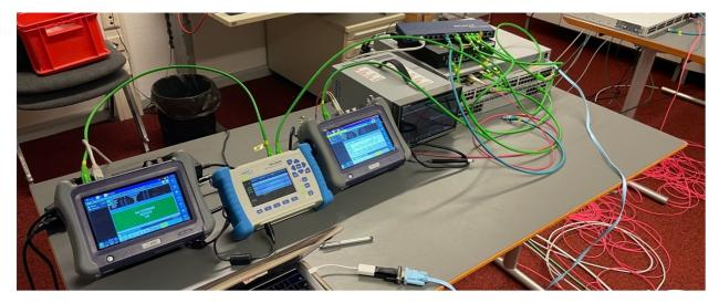
From left to right: MTS-5800 (PTP-Server) -> WAN emulator -> distribution switch -> Boundary Clock switches under test
