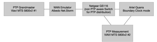
The Quarra switch was locked and stabilized over several minutes. Its proper lock status to the PTP grandmaster was verified by analyzing its announce messages using Wireshark. Additionally, the re-distributed PTP time the switch under test was compared to GPS as the global reference.
