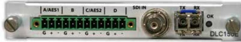
**Figure 9.** DLC150E Audio, Electrical, and SFP Optical Connectors
