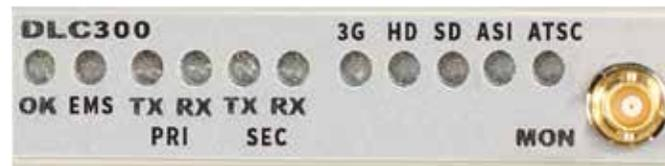
**Figure 7. DLC300 Front Panel Status LEDs and Monitor Connector**
