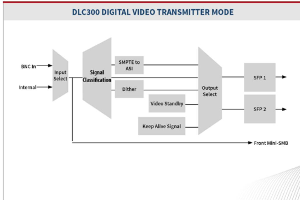
**Figure 1. DLC300 Module Functional Block Diagram**
