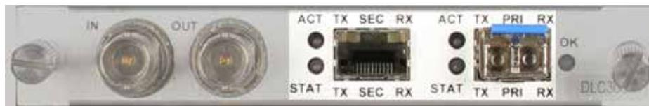
**Figure 8. DLC300 Rear Panel Status LEDs**
