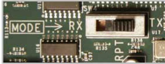
**Figure 3.** DLC300 SW4 Mode Select Switch
