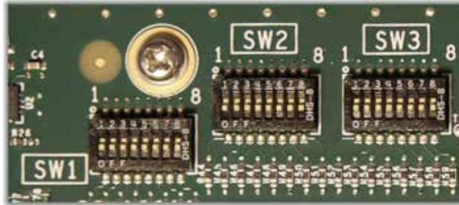
**Figure 4. Configuration DIP Switches**
