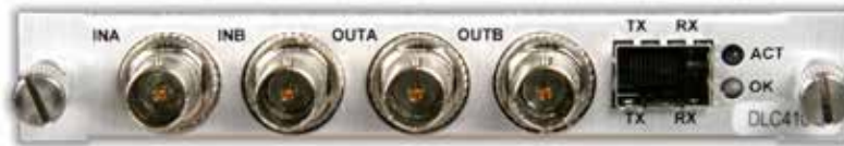
Figure 5. DLC410 BNC Connectors and SFP Socket
