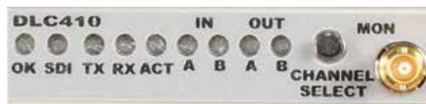
Figure 6. DLC410 Status LEDs and Monitor Connector
