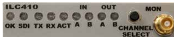
Figure 6. ILC410 Status LEDs and Monitor Connector
